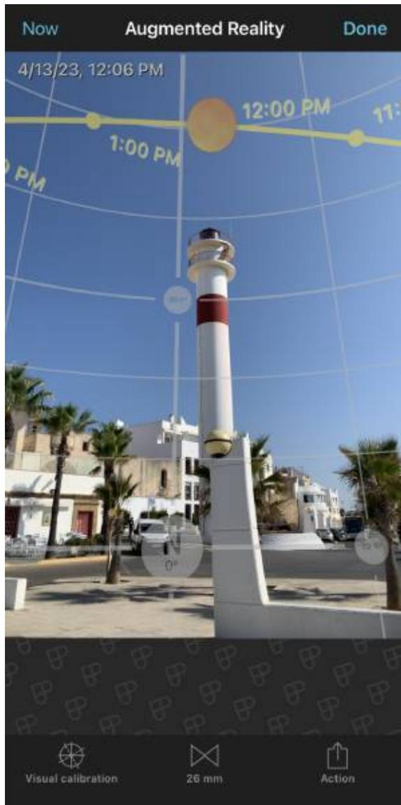
PhotoPills Sun Pill Augmented Reality view - It gives you the position and path of the Sun for the selected location (by default where you are), date and time (by default the current ones).
