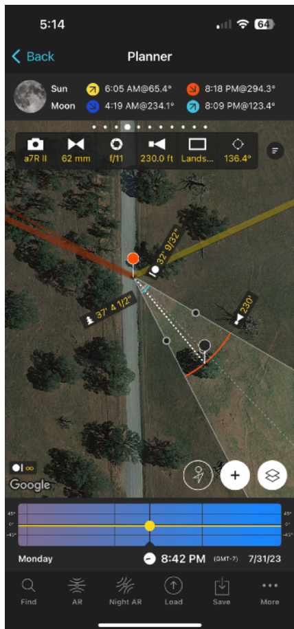
Left - PhotoPills plan for Spenceville Wildlife Area on 7/31/23. Camera is Sony a7rii, Focal Length 62mm, F-stop 11. Focus Distance 230 feet (Subject Tree) and DoF from 32 feet in front of camera out to Infinity.
